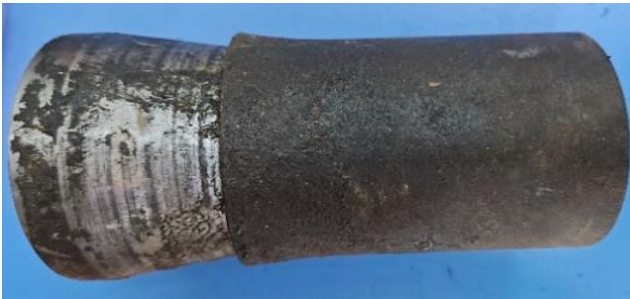
Fig. 1. Expansion cone and pipe
